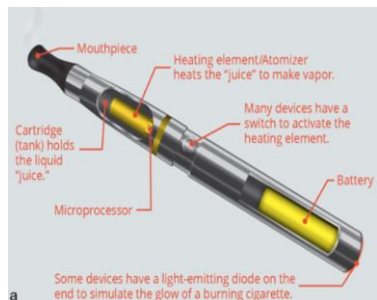
Figure 1. Diagram of E-cigarette components
